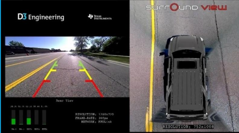
A 4-camera system that gives a 360° view; capable of stitching feeds together to generate a 3-dimensional, real-time rendering of the vehicle's surroundings.
